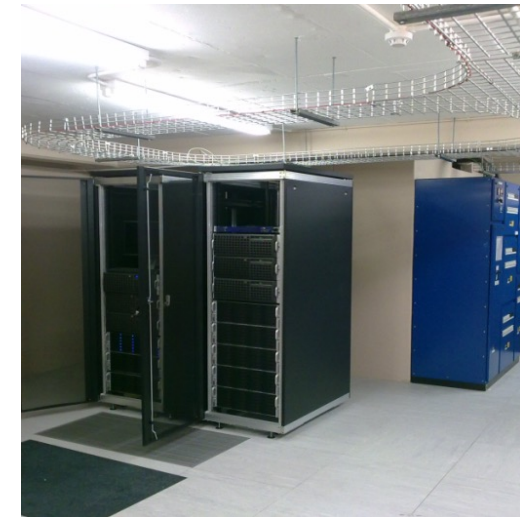
2010: GPU Cluster; 2.4 GHz; 96 cpu cores; 22 GPU's 16 Tflops ; 14 TB file system
