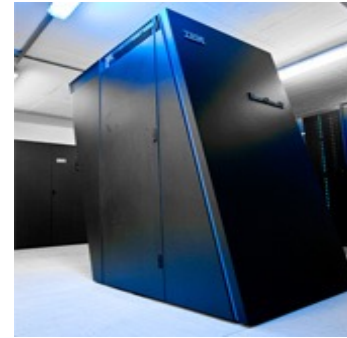
2008: IBM Blue Gene/P; 0.8 GHz; 4096 cores; 11.5 Tflops
